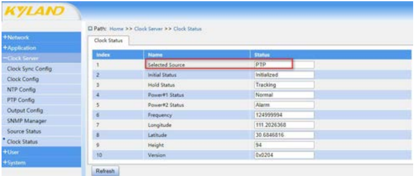
Figure 38 Current Synchronization Source PTP
