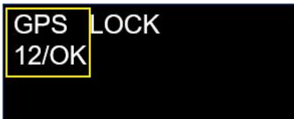
Figure 74 Synchronization source status: GPS
