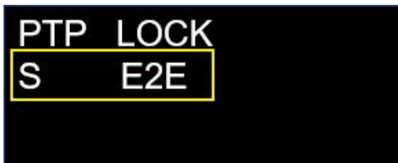
Figure 78 Synchronization source status: PTP Slave clock, E2E
