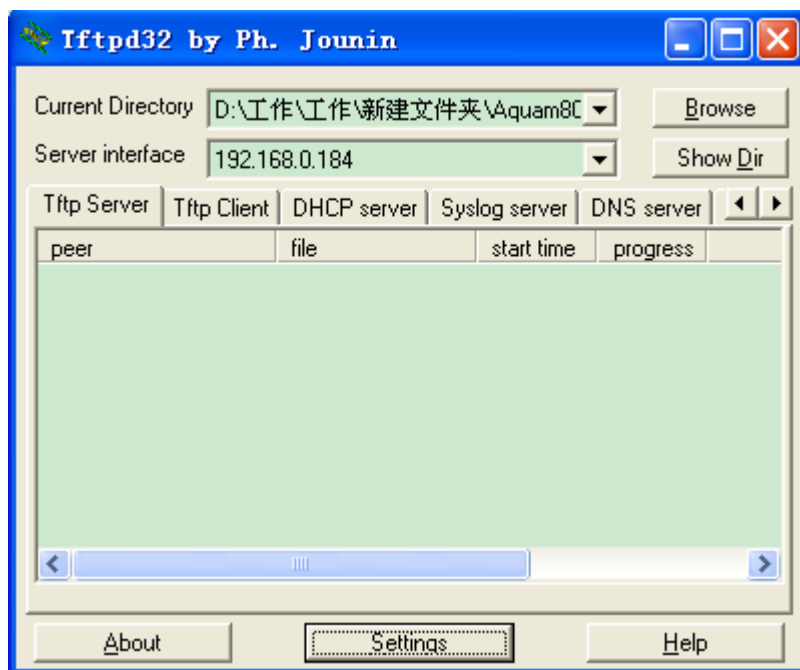
Figure 80 TFTP Server Configuration
